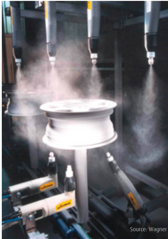
Figure 1: Powder coating of aluminium wheels
